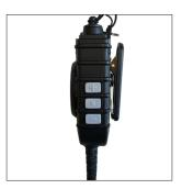
Volume +/- buttons and loudspeaker on/off switch when headset connected.
